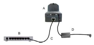
Figure 6 - Ethernet Connection
